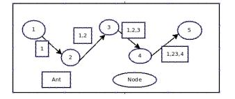
**Figure. 1**: Ant traversing the network and providing routing information to nodes
